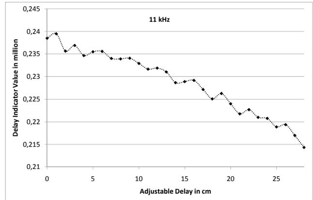
Fig. 13. The figure shows the delay value indicator when employing two 11 kHz localization signals. The data points results from varying length of the employed line stretcher.
