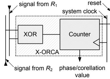
Fig. 3. An X-ORCA phase detector consists of a logical XOR (or any other suitable binary logic function), which “mixes” the two input signals  $s_1$  and  $s_2$ , and an additional counter to actually determine the phase shift  $\Delta\varphi$ .
