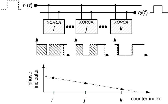
Fig. 4. X-ORCA places all phase detectors along two reciprocal (anti-parallel) “delay” wires  $w_1$  and  $w_2$  on which the two signals  $r_1(t)$  and  $r_2(t)$  travel with approximately two third of the speed of light  $c_w \approx 2/3c$ . Because the two wires  $w_1$  and  $w_2$  are *reciprocal*, all phase detectors have different internal delays  $\tau_i$ .
