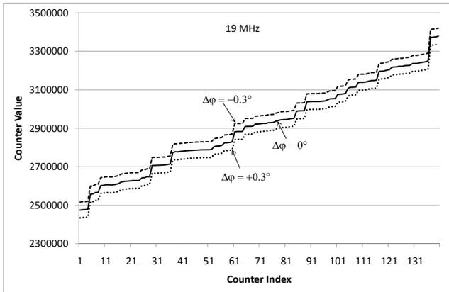
Fig. 8. This figure shows the counter values  $v_i$  of  $n = 140$  phase detectors when exposed to two 19 MHz signals with zero phase shift  $\Delta\varphi = 0$  (solid line), with phase shift  $\Delta\varphi \approx -0.3^\circ$  (dashed line), as well as with phase shift  $\Delta\varphi \approx +0.3^\circ$  (dotted line).
