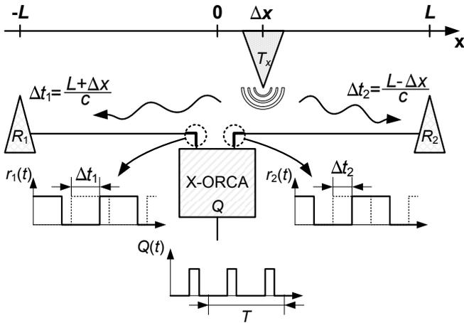
Fig. 2. X-ORCA assumes a standard, one-dimensional setup in which the time difference  $\Delta t = t_1 - t_2 = 2\Delta x/c$  is a result of the transmitter's off-center position  $\Delta x$ . It indirectly determines  $\Delta t = \Delta\varphi/(2\pi f)$  by estimating the phase shift  $\Delta\varphi$  between the two incoming signals  $r_1(t)$  and  $r_2(t)$ .
