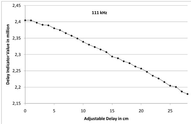
Fig. 12. The figure shows the delay value indicator when employing two 111 kHz localization signals. The data points results from varying length of the employed line stretcher.
