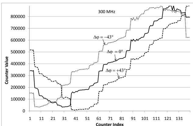
Fig. 9. The figure shows the counter values  $v_i$  of  $n = 140$  phase detectors when fed with two 300 MHz signals with zero phase shift  $\Delta\varphi = 0$  (solid line), with a phase shift  $\Delta\varphi = -43^\circ$  (dotted line), as well as with a phase shift  $\Delta\varphi = +43^\circ$  (dashed line).
