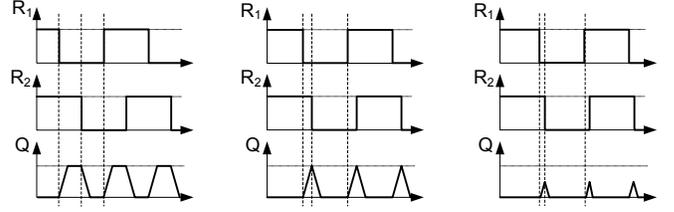
Fig. 5. Due to the inherent rise and fall times, a change in a gate’s output requires some time. Therefore, if the input frequency increases too much or if the input edges come too close together, the gate cannot properly change its output (right-hand-side).
