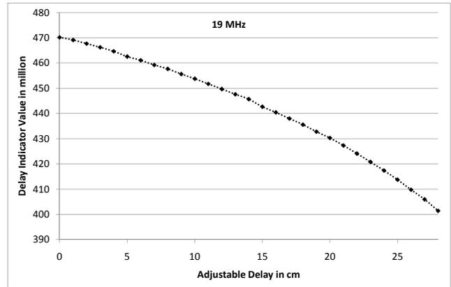
Fig. 10. The figure shows the delay value indicator when employing two 19 MHz localization signals. The data points results from varying length of the employed line stretcher.
