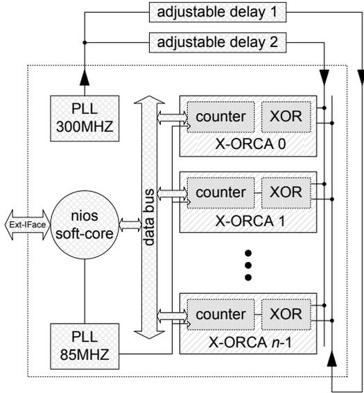
Fig. 6. On the top-level, the X-ORCA implementation consists of 140 phase detectors (aligned from top to bottom), a Nios II processor, a first PLL for the system, a second PLL for the localization signal with a frequency of 300 MHz, and just a little bit of additional infrastructure.
