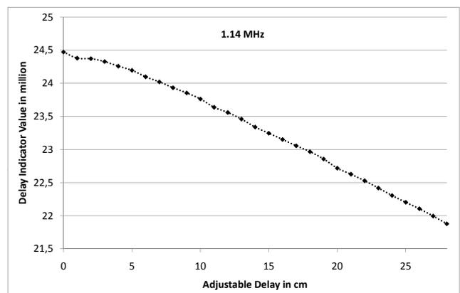
Fig. 11. The figure shows the delay value indicator when employing two 1.14 MHz localization signals. The data points results from varying length of the employed line stretcher.
