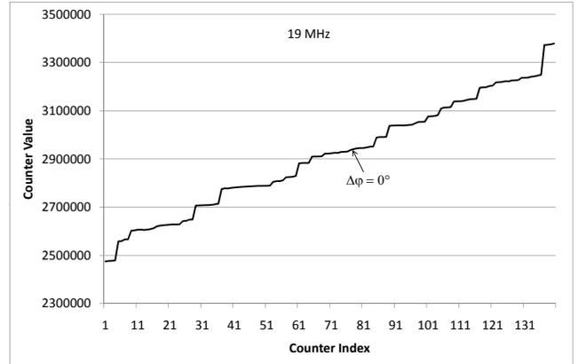
Fig. 7. This figure shows the counter values  $v_i$  of  $n = 140$  phase detectors when exposed to two 19 MHz signals with zero phase shift  $\Delta\varphi = 0$ .
