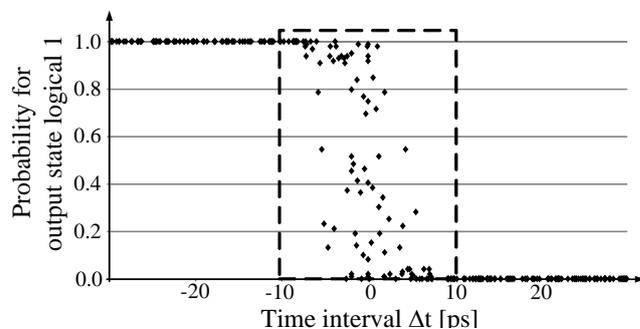
Fig. 9. Illustration of transient area of all BOUNCE elements. All elements fully change their output behavior within 20 ps (dashed line).
