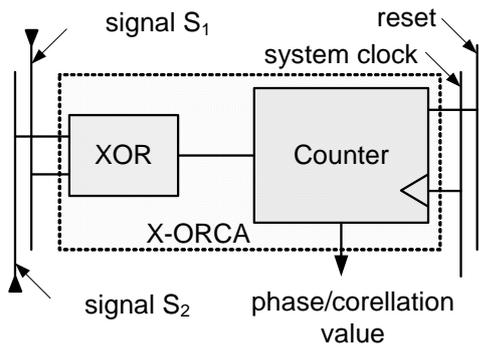
Fig. 6. Schematic of the original X-ORCA phase detector.
