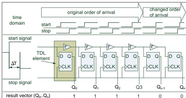
Fig. 1. Basic principle of operation of a Tapped Delay Line (TDL)
