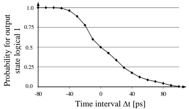
Fig. 5. Output probability for one single BOUNCE element, caused by calibration side effects and internal behavior of the flip flop.
