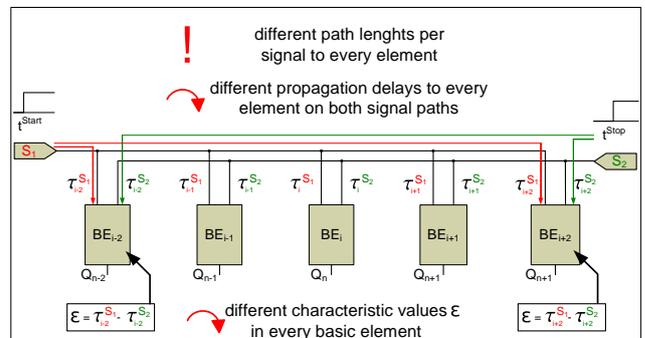
Fig. 2. The BOUNCE approach: placing latches at different positions to yield different propagation delays.
