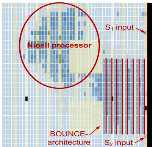
Fig. 3. On-Chip layout of BOUNCE: 1024 detectors are placed in the right side of the chip. Picture taken from Alteras FPGA synthesis tool.
