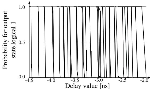
Fig. 8. Results of first experiment, every curve corresponds to one BOUNCE element. Every single element changes its output value at a certain delay.
