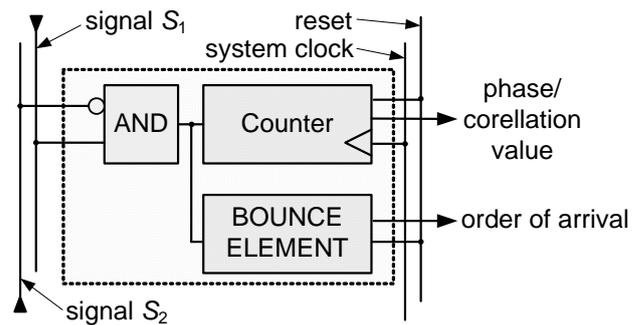
Fig. 7. Schematic of the combined X-ORCA/BOUNCE element. Notice the modified signal entry gate.
