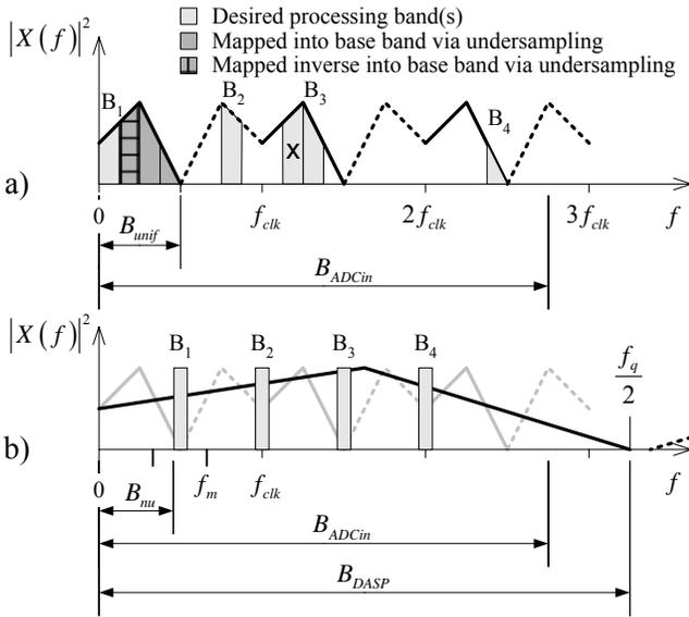
Fig. 1: Traditional undersampling a) versus DASP-sampling b) avoiding aliasing. Processing bands may be chosen such that arbitrary periodic signals can be analyzed.
