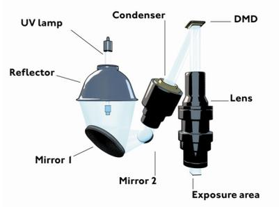
**Figure 13: Optical system of the UV-Setter, courtesy of Punch Graphix Prepress Germany, Ltd.**
