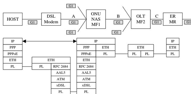
Figure 8: Access Network with MF in ONU and OLT
