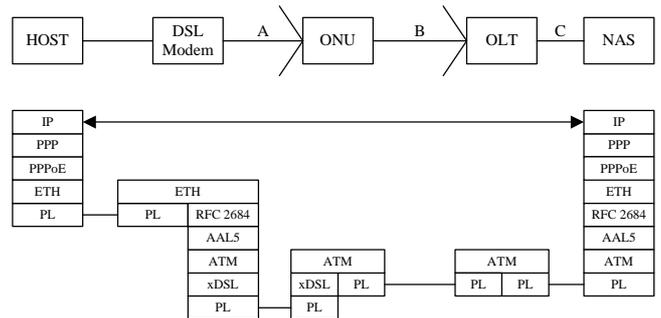
Figure 3: Access Network - ATM Based
