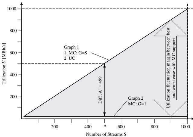
Figure 5: Utilisation of a Gigabit Ethernet
