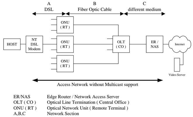
Figure 2: General Structure of an Optical Access Network
