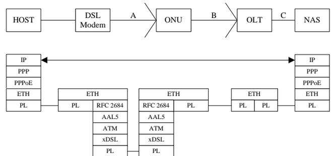
Figure 4: Access Network - Ethernet Based
