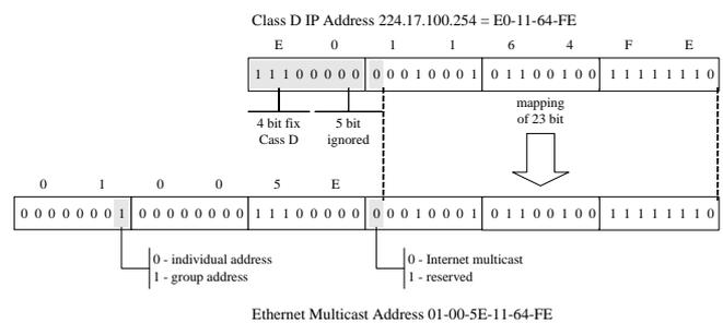
Figure 1: Mapping of IP to Ethernet Multicast Addresses
