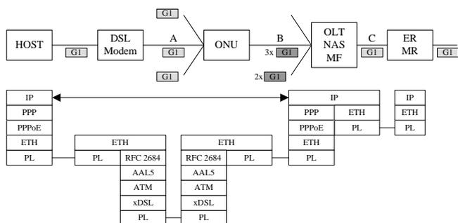
Figure 7: Access Network with MF inside OLT
