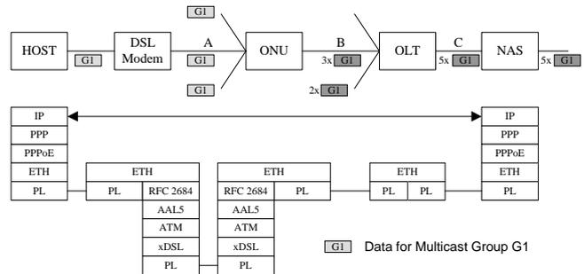
Figure 6: Ethernet Based Access Network without MF
