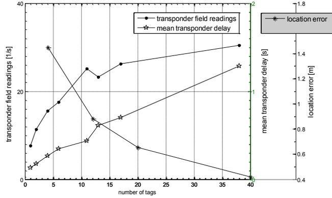
**Figure 3.** Mean readings, mean delays and mean location error for changing transponder numbers
