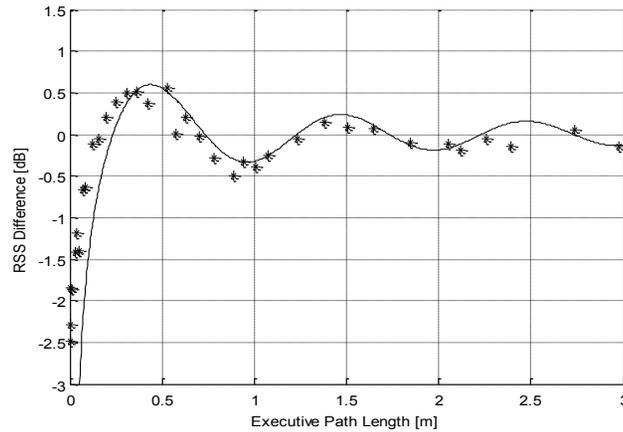
**Figure 1.** Theoretical model regression and experimental data points from multiple transponder scenario
