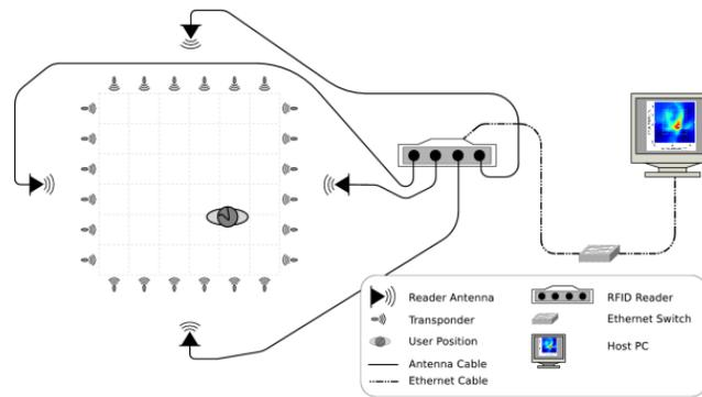
**Figure 5.** Experimental setup and system structure
