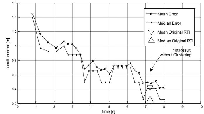
**Figure 8.** Positioning error progression with constant clustering rate
