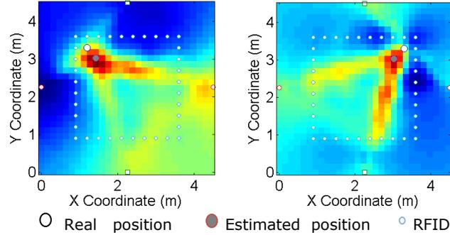
**Figure 2.** Passive RFID Tomographic Images
