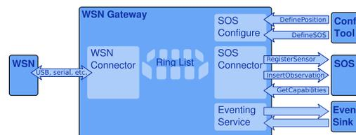
Figure 7. WS4D Sensor Web Gateway implementation
