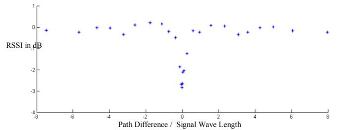
Fig. 3. Median RSS Indicator for relative User Positions [8]
