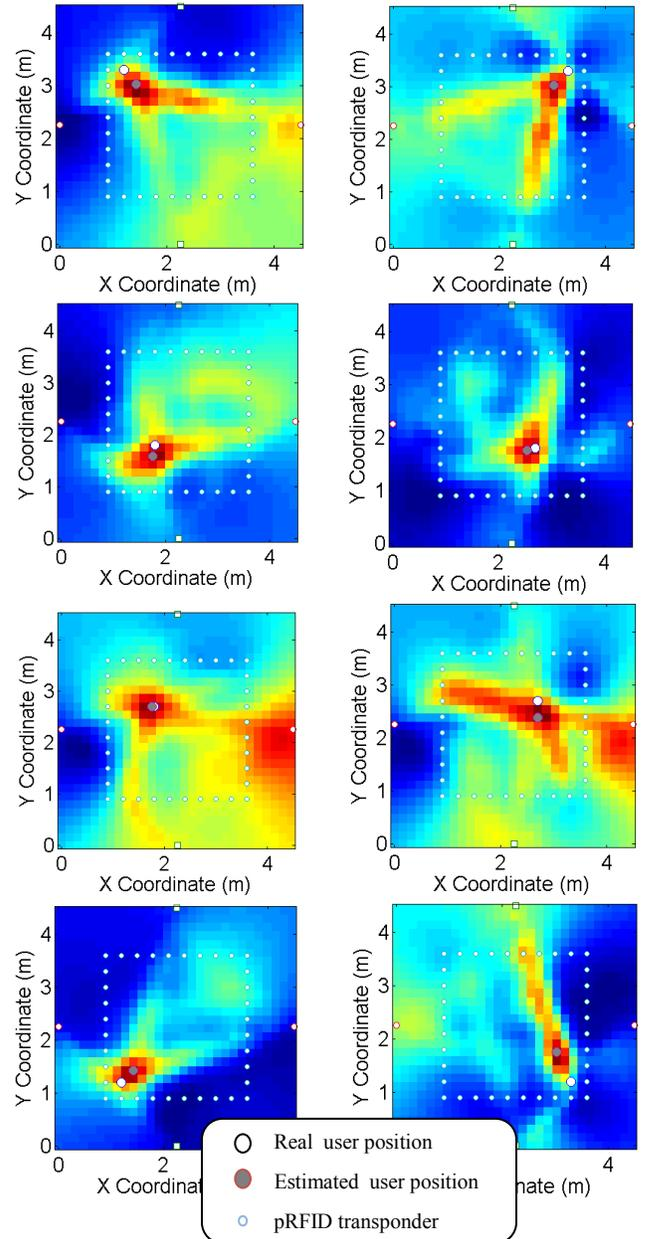
Fig. 8. Example resulting images for pRFID based tomography
