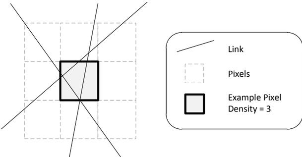
Fig. 5. Link density definition example for one pixel
