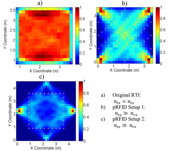
Fig. 6. Link density images based on the original RTI setup and two different pRFID setups
