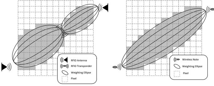
Fig. 4. Adaptive pixel weighting with a sensor node network (right) compared to bistatic pRFID (left)
