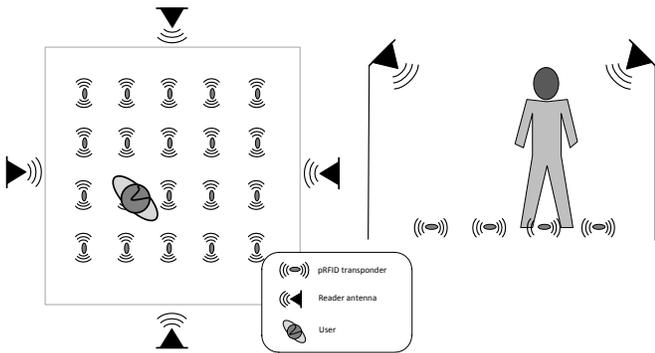
Fig. 2. Setup of the new pRFID based DFL approach
