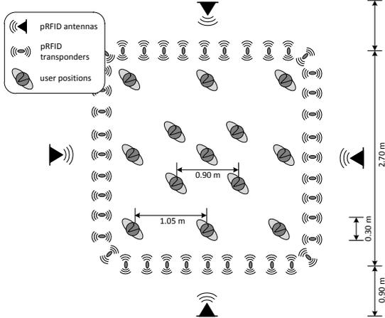
Fig. 7. Experimental pRFID setup for validation
