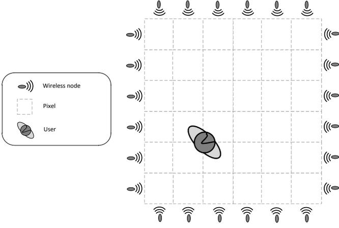
Fig. 1. Setup of a standard Radio Tomographic Imaging deployment
