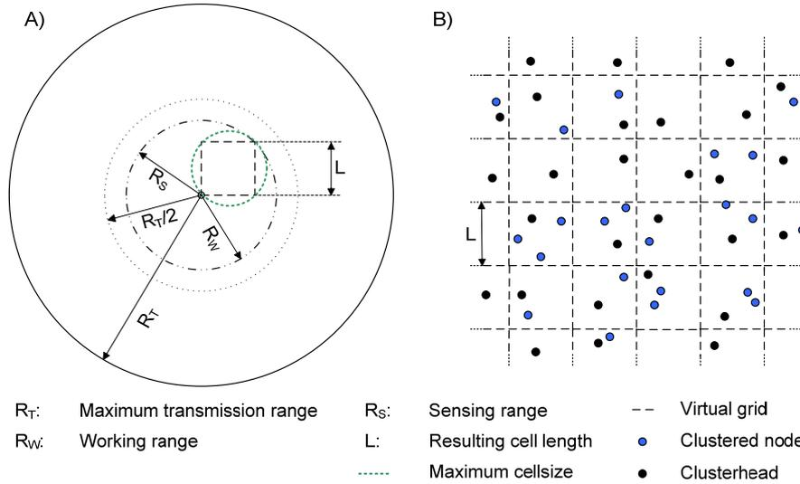
Figure 1: XGAF approach A) Estimation of maximum square cell sizes B) Appliance to a WSN with random distributed nodes
