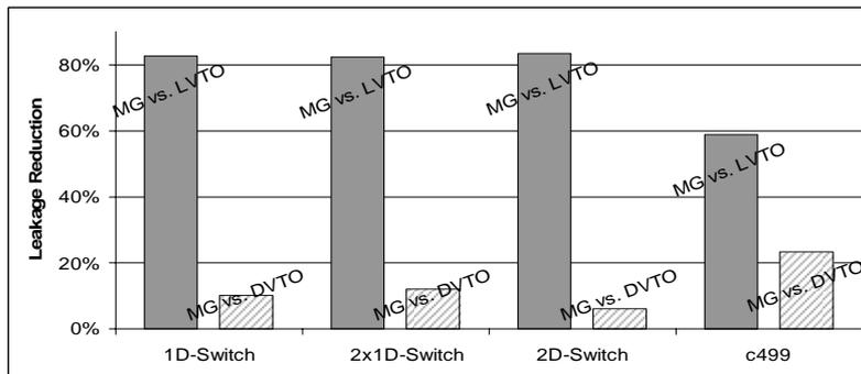
**Figure 6. Achieved reduction of leakage currents for the Mixed Gates approach compared to LVTO and DVTO designs**
