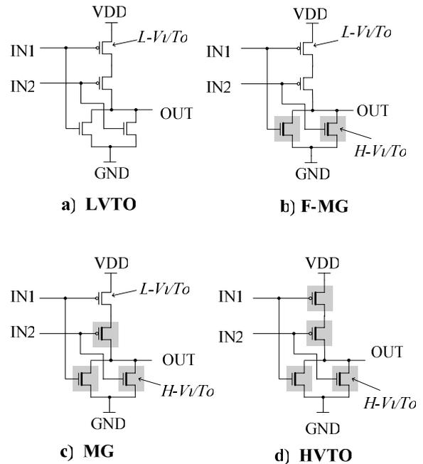
**Figure 2. Different implementations of a NOR2 gate: LVTO, HVTO, and Mixed Gates**
