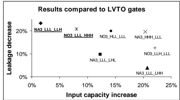
Figure 4. Different implementations of F-MG for a 3-input NAND (NA3) and NOR (NO3) gate
