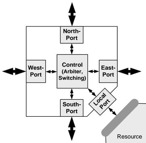
Figure 5. Basic structure of a 2D switch with five ports for dimension-ordered routing
