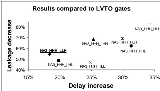
Figure 3. Comparison of possible MG realizations for a NAND3 (NA3) gate
