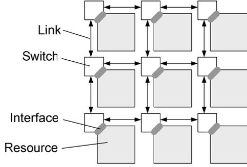
**Figure 1. Basic structure of 3x3 Network-on-Chip with a mesh topology**
