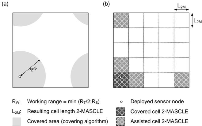
Fig. 5. Simulation area without edge conflicts a) Covering algorithm b) 2-MASCLE
