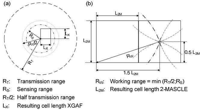
Fig. 1. Calculating the resulting cell length of a) XGAF cell. Resulting cell length guarantees connectivity to adjacent and diagonal adjacent nodes and complete cell coverage by a member node b) 2-MASCLE cell. Resulting cell length allows complete coverage by adjacent nodes and a transmission to one cell above the next adjacent node in a row.
