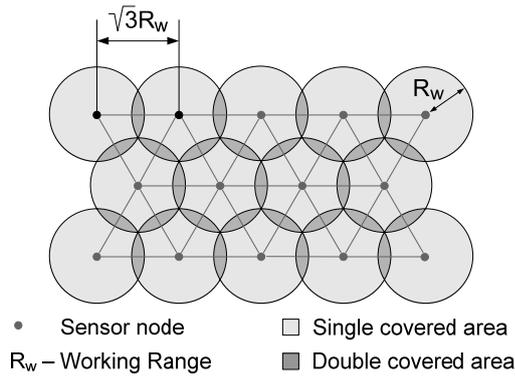
Fig. 12. Deployment of sensor nodes as edges of equilateral triangles for maximum efficiency
