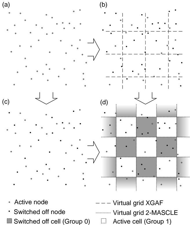
Fig. 3. Development of 2-MASCLE a) Sensor node field with randomly distributed nodes b) Applied XGAF algorithm c) Applied 2-Covering algorithm d) Applied 2-Mascle
