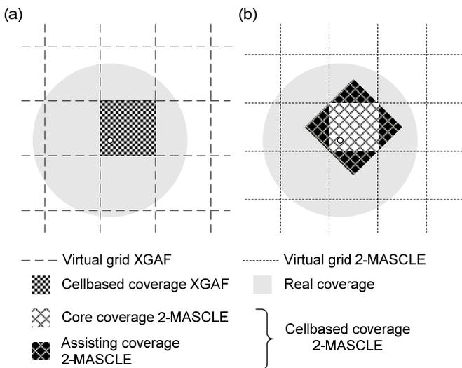
Fig. 6. Real coverage of a node versus simplified cell based coverage of a) an XGAF cell b) a 2-MASCLE cell
