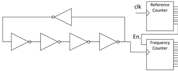
Fig. 1. Schematic of a ring oscillator and frequency counter, which is enabled by a reference counter
