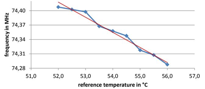
Fig. 4. Linear relationship between temperature and oscillation frequency
