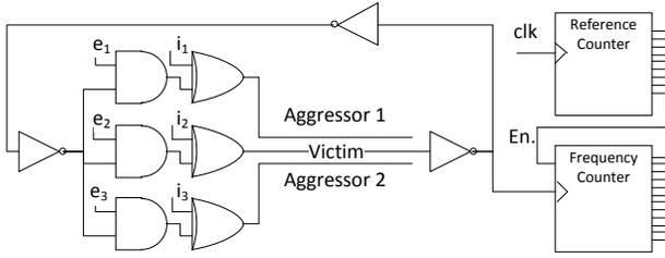
Fig. 2. Schematic of a measurement circuit for crosstalk induced delay
