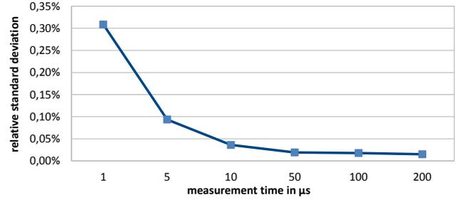
Fig. 3. Relative standard deviation of frequency measurements at a specific temperature over different time spans of measurement
