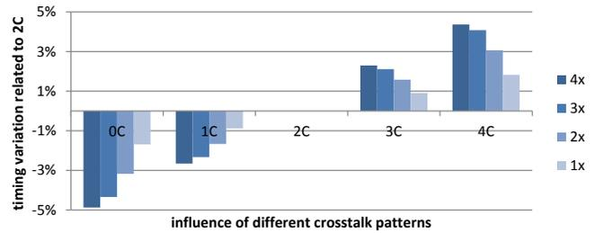
Fig. 5. Crosstalk induced delay for Virtex 6 normalized to pattern 2C
