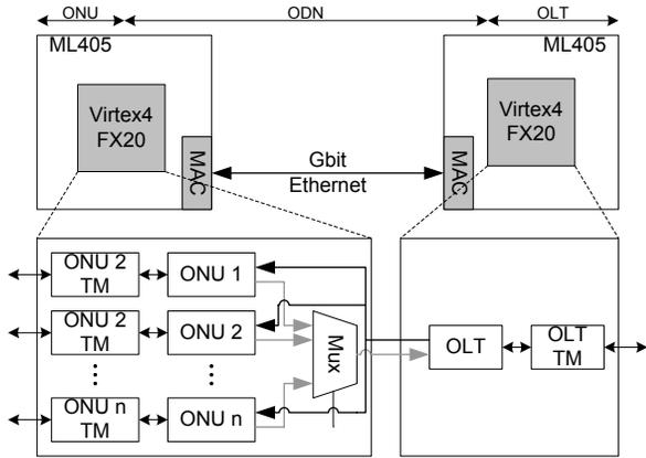
**Figure 6. Prototype architecture of the evaluation platform**
