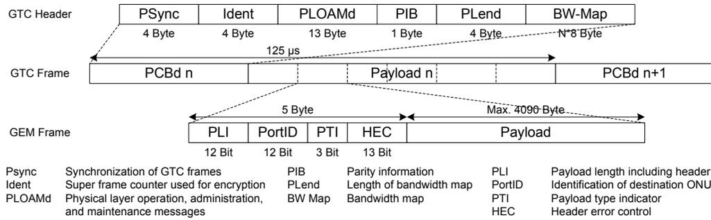
Figure 3. Frame structure of a downstream GTC frame
