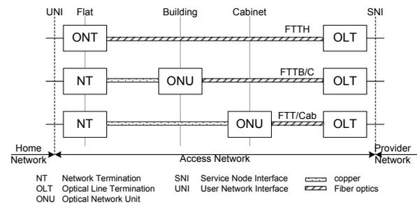
Figure 1. FTTx network architectures
