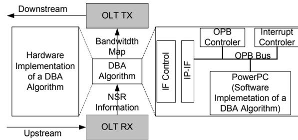
**Figure 8. Hard- and software DBA algorithm implementation**
