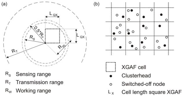
Figure 1. Square XGAF algorithm (a) Estimation of the maximum cell size (b) Application to a sensor network
