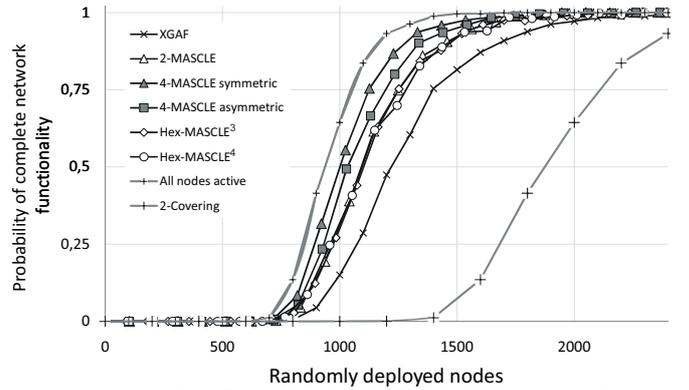
Figure 7. Probability of complete network functionality versus randomly deployed nodes
