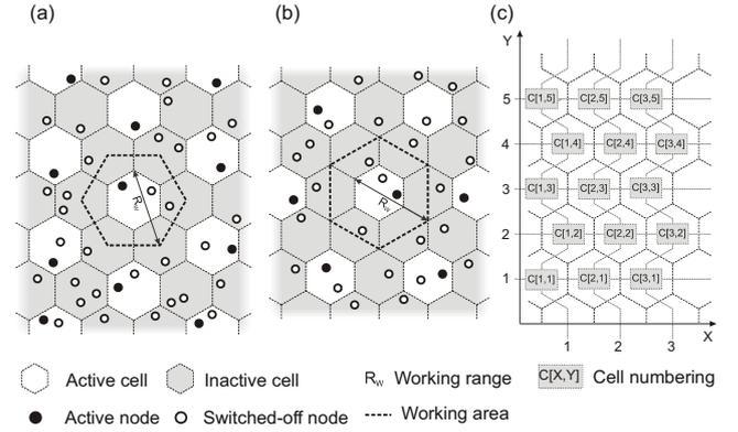
Figure 3. Hexagon MASCLE algorithm (a) Version with 3 phases (b) Version with 4 phases (c) Cell numbering
