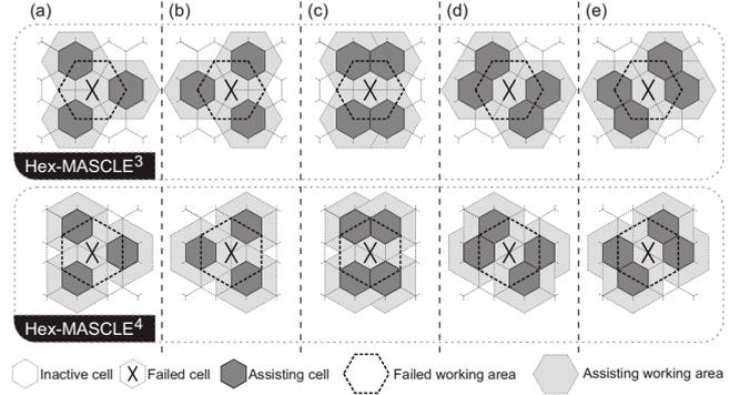
Figure 5. Assistance in Hexagon-MASCLE (a-b) with 3 adjacent cells, (c-e) with 4 adjacent cells. From left to right: Preferred assistance arrangements
