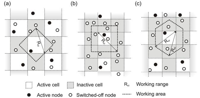
Figure 2. Applied MASCLE-algorithms (a) 2-MASCLE (b) Symmetric 4-MASCLE (c) Asymmetric 4-MASCLE
