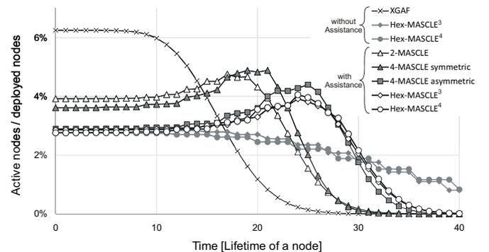
Figure 8. Active nodes versus runtime of the network
