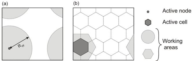
Figure 6. Simulation area without edge effects. Working area of (a) a single sensor node, (b) Hex-MASCLE<sup>3</sup>
