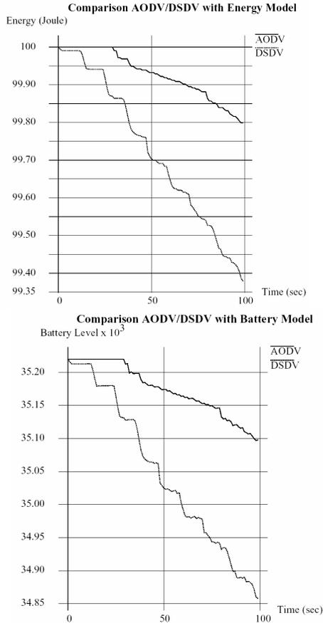
**Fig. 8:** Simulation of Ad-Hoc Routing Protocols AODV and DSDV with Energy Model (above) and Battery Model (below).
