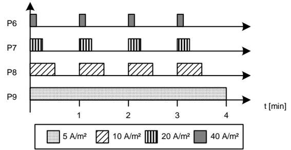
**Fig. 5:** Discharge Profiles for Battery Lifetime Estimation.
