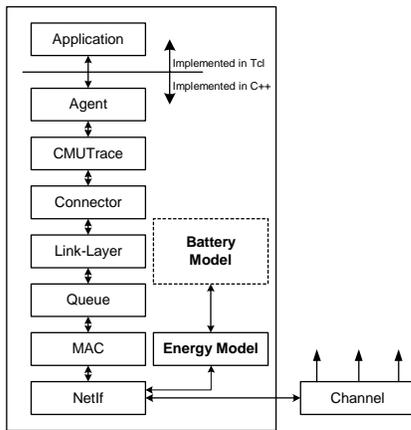
**Fig. 6:** Block Diagram of an NS2 Mobile Node with Battery Model
