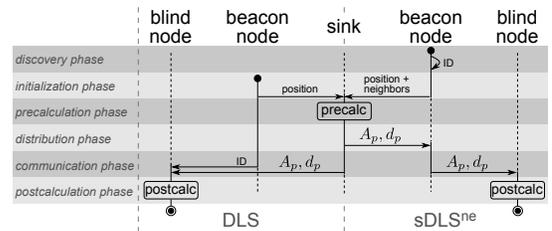
Figure 1. Algorithmic comparison of DLS and sDLS<sup>ne</sup>
