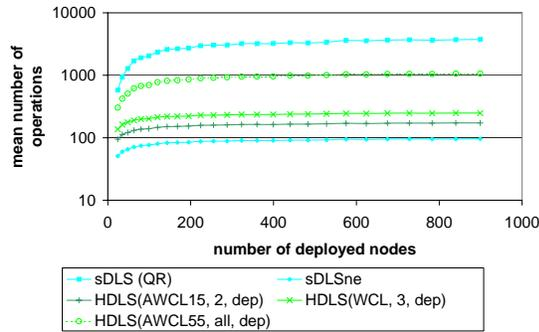
Figure 19. Mean number of operations of best performing HDLS approaches for different limits of virtual beacon nodes
