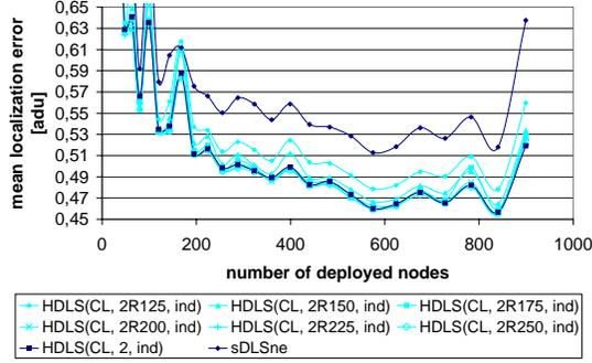
Figure 11. Mean localization error of CL based HDLS with independent distance estimation and range based virtual beacon strategy
