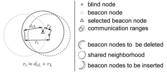
Figure 3. Approximation of a distance between blind node and inaccessible beacon node  $i$  by means of the linearizing beacon node  $L$
