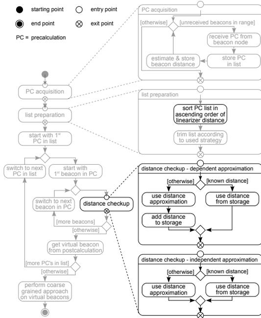
Figure 5. Differences of independent and dependent distance approximation (left), illustrated in the context of the HDLS algorithm (right).
