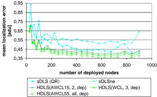
Figure 17. Mean localization error of best performing HDLS approaches for different limits of virtual beacon nodes
