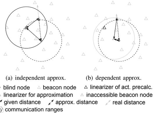
Figure 4. Two approximation strategies: To estimate distances of inaccessible beacon nodes, included in a precalculation, either (a) the beacon node, providing the precalculation or (b) the closest beacon node is used.
