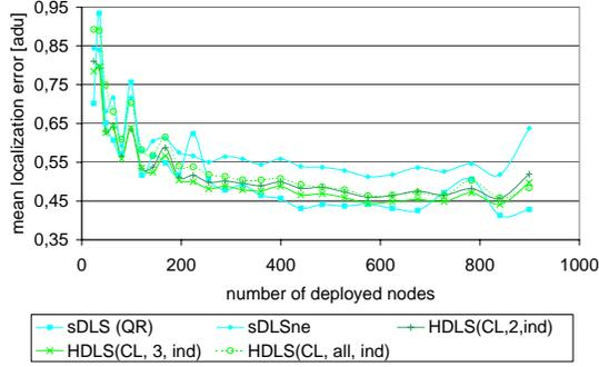
Figure 7. Mean localization error of CL based HDLS with independent distance estimation
