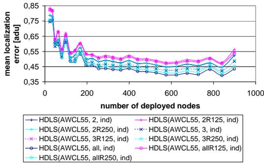
Figure 12. Mean localization error of AWCL based HDLS with independent distance estimation and range based virtual beacon strategy
