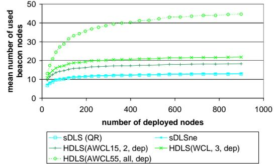
Figure 18. Mean number of used beacon nodes of best performing HDLS approaches for different limits of virtual beacon nodes
