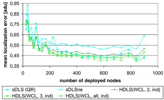
Figure 8. Mean localization error of WCL based HDLS with independent distance estimation
