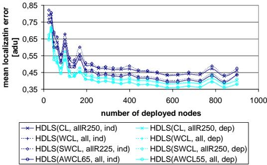
Figure 16. Mean localization error of best performing HDLS approaches, grouped by estimation technique and distance approximation
