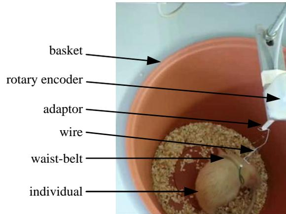
Figure 1: Experimental Setup for Rotation Tests based on a wired connection from rat to decoder
