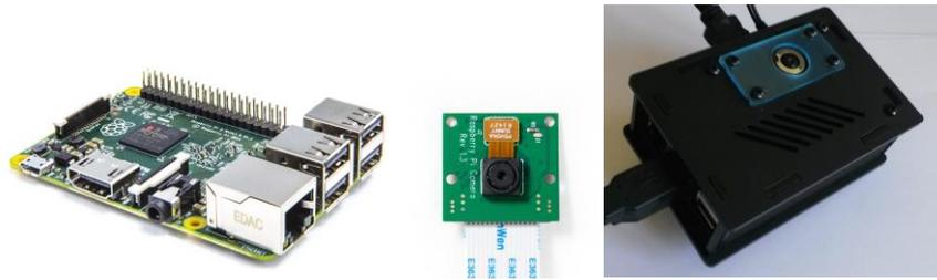
Figure 2: Raspberry Pi Development Board, Raspicam, and Nwazet Pi Camera Box (from left to right)
