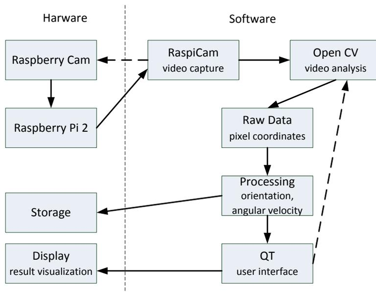
Figure 3: Structural System Overview: Functional Separation in Hardware and Software Components
