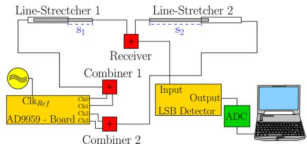
Fig. 2. Schematic diagram of the laboratory setup. All wire-pairs have the same lengths between the AD9959-Board and the Receiver for the both transmissions lines.
