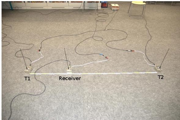
Fig. 3. Radio-based setup with the two transmitters (T1 and T2) and the receiver between them.
