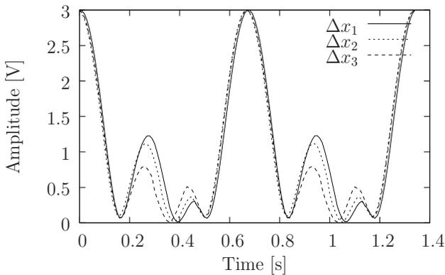
Fig. 1. Three real measured LSB periods (scaled positive envelope to 3V). The LSB period ranges from about 0.5s to 1.16s. The length is equal to  $1/\Delta f$  for the dedicated values of the experiment.
