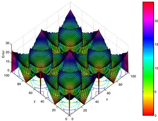
**Figure 2. Error distribution over an array of  $3 \times 3$  beacons, transmission range=50, array width=100. The beacons are arranged as in Fig. 1.**
