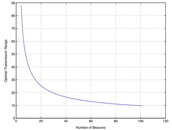
**Figure 10. a) Dependency of positioning error on number of beacons and transmission range, b) Optimal transmission range over number of beacons,  $101 \times 101$  nodes at array width=100**
