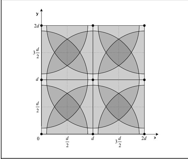
**Figure 4. Four overlapping regions in an array of 3x3 beacons with transmission range  $r_{\min} < r < r_{\max}$**
