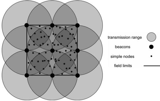
**Figure 1. Overlapping regions in a 3×3 array with 9 beacons and 68 randomly distributed sensor nodes.**
