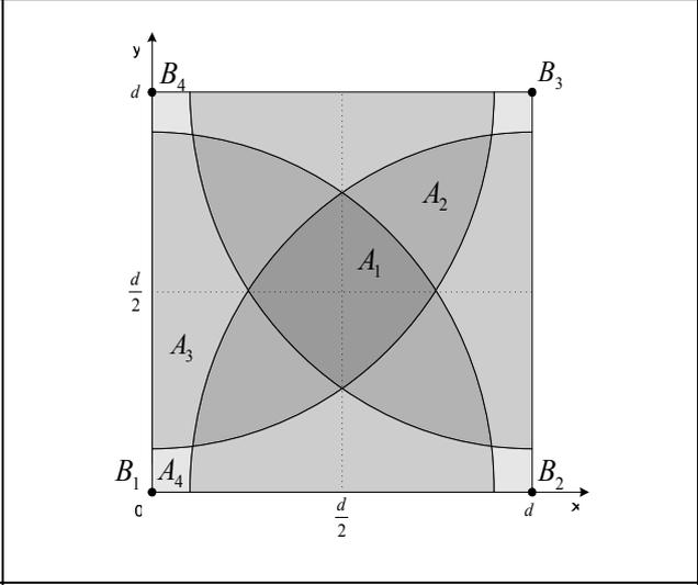
**Figure 5. One overlapping region A enclosed by beacons  $B_1 \dots B_4$  and subdivided into regions  $(4 \cdot A_1, 4 \cdot A_2, 8 \cdot A_3, 4 \cdot A_4)$**
