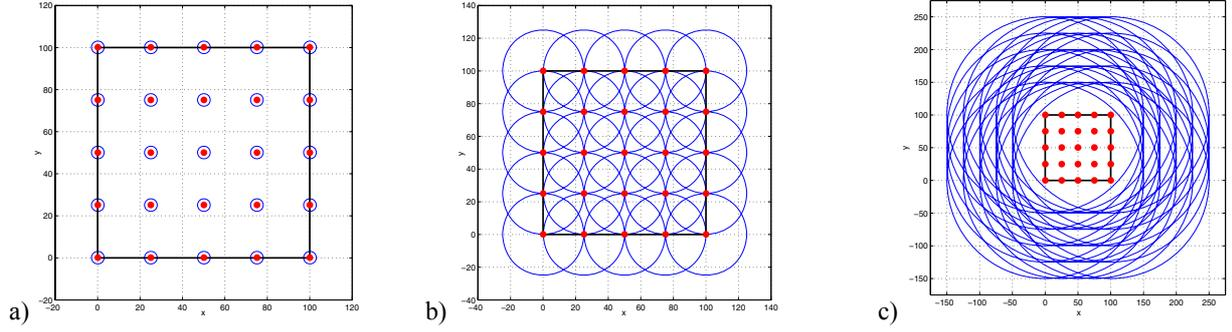
**Figure 3. Three scenarios showing a finite wireless sensor network within the solid rectangles consisting of randomly distributed sensor nodes (not shown) and 5×5 beacons with a) low, b) optimal, c) high transmission ranges. In all cases, sensor nodes determine their own position based on positioning information received from neighboring beacons.**
