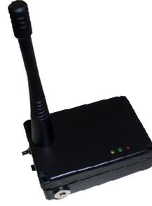
Fig. 3. Encapsulated evaluation module CC1010EM in a chassis with additional hardware and batteries to work autonomously.
