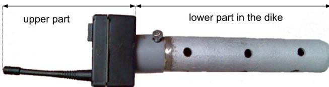
Figure 2. Sensor node equipped with a CC1010 evaluation module from Texas Instruments as upper part and a metal pipe containing the circuit to detect the water level as lower part.
