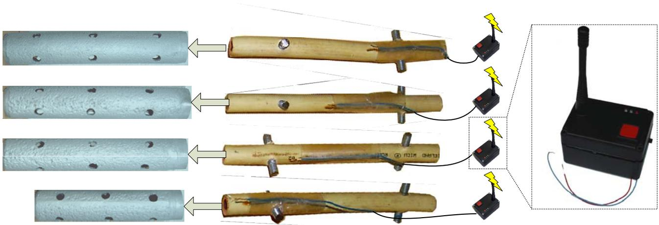
Figure 5. The node consist of a circuit that is mounted on an inner pipe. The inner pipe is moved into the outer pipe, which is made of solid metal and protects the circuit. The wiring of the inner circuit is connected to the pins of the sensor node.
