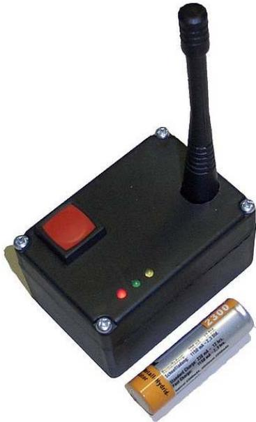
Figure 1. Encapsulated CC1010 sensor evaluation module.
