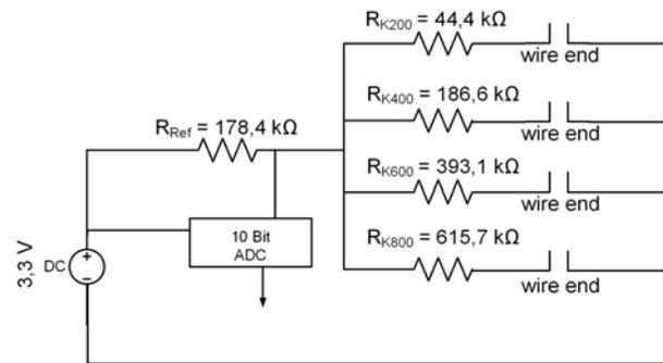
Figure 3. Circuit to detect the water level in the outer pipe.
