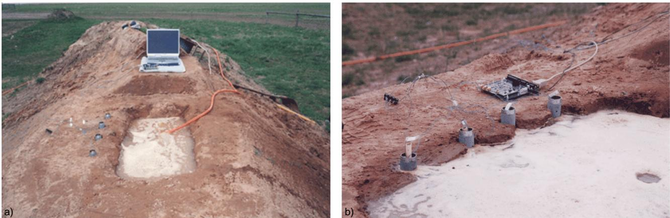
Figure 7. a) Artificial dike with four nodes (here without mounted CC1010 evaluation module on every pipe); b) Water has already eroded the surface and the dike threatens to break.
