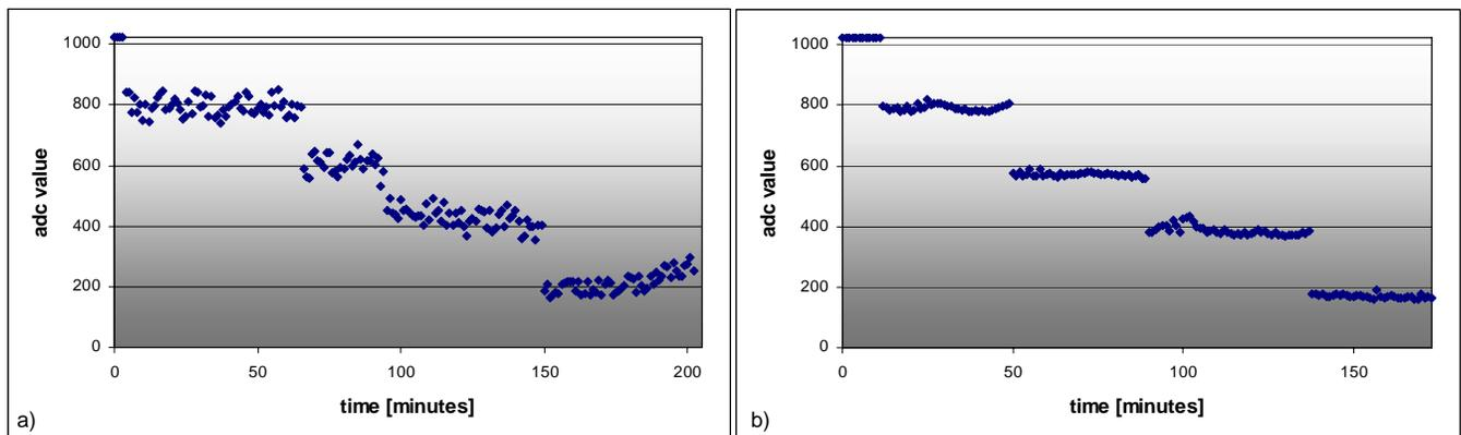
Figure 6. Measurements of the voltage over the reference resistor to detect a) pure sweet water and b) 11% pure salt water, which slowly floods the outer pipe.
