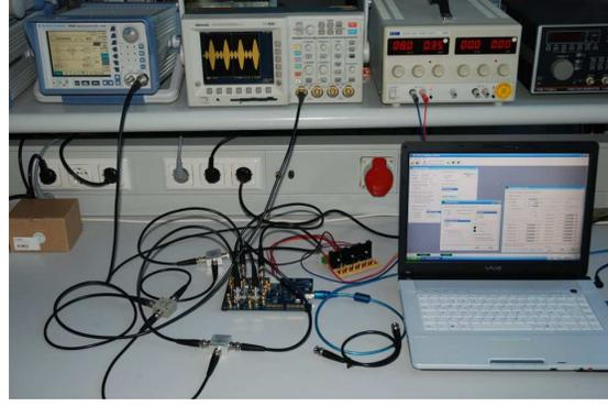
**Figure 5.** The left-hand-side shows the schematically the setup of the experiment in which a DDS-Chip AD9959 generates four reference signals. Two mini-circuit combiners ZFSC-2-1 generate the actual beats  $b_1(t)$  and  $b_2(t)$ . A third combiner simulates a receiver and displays its signal readings  $r_{\Delta x}(t)$  on a Tektronix TDS 3034 oscilloscope. The right-hand-side shows the actual laboratory equipment.
