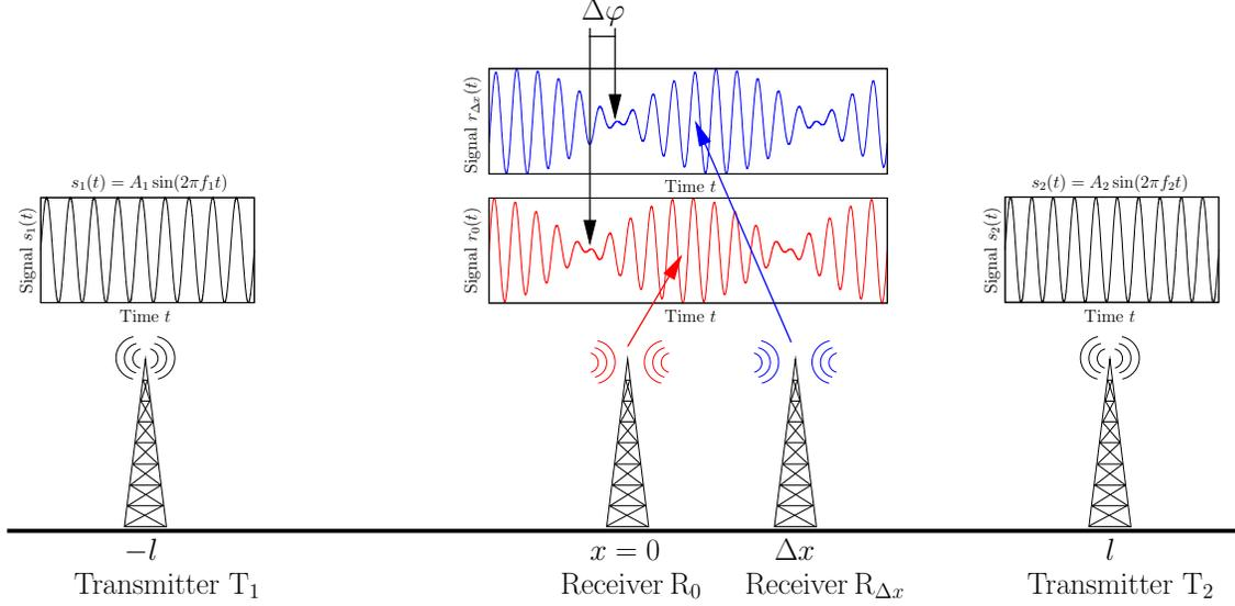
**Figure 1.** This analysis assumes a setup with two transmitter  $T_1$  and  $T_2$  as well as two receivers  $R_0$  and  $R_{\Delta x}$  that are located at  $x = -l$ ,  $x = l$ ,  $x = 0$  and  $x = \Delta x$ , respectively. The figure also shows that both receivers sense a beat with a location-dependent phase-shift  $\Delta\varphi$ .
