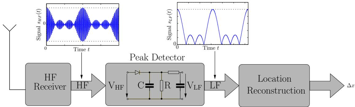
**Figure 7.** This figure shows a block diagram for the detector.
