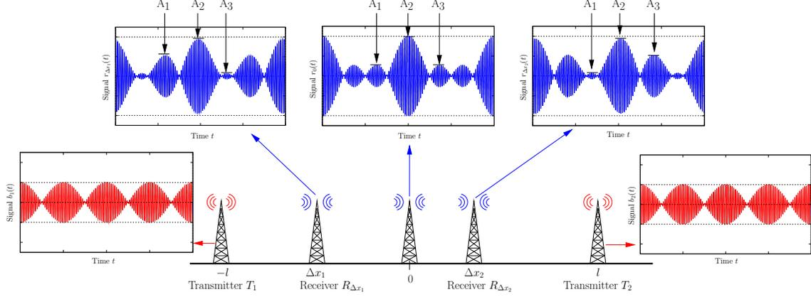
**Figure 2. The superposing-beats procedure: two transmitter  $T_1$  and  $T_2$  emit modulated signals  $b_{1/2}(t) = A_{1/2} \sin(2\pi f_{1/2}t) \cos(2\pi f_m t)$  as well as two receivers  $R_{\Delta x_1}$  and  $R_{\Delta x_2}$ . The figure clearly shows that the two modulated carrier signals induces location-dependent interference patterns.**
