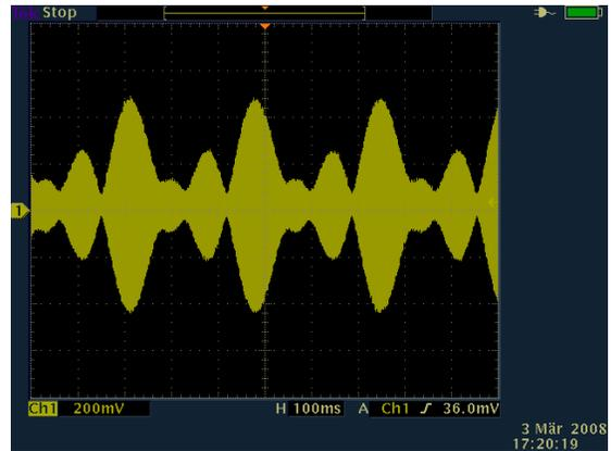
**Figure 6.** This figure shows the signals  $r_{\Delta x}(t)$  a receiver would read at the four distance differences  $\Delta x \approx 0$  cm,  $\Delta x \approx 50$  cm,  $\Delta x \approx 100$  cm, and  $\Delta x \approx 150$  cm.
