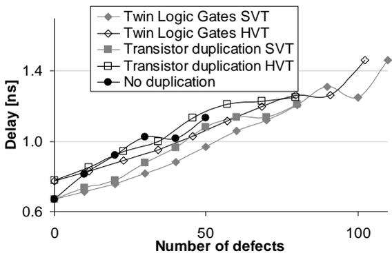
Figure 7 Average Delay for the basic multiplier and the multipliers with gate and transistor duplication
