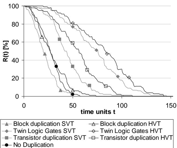
Figure 5 Comparison of simulated results for the reliability of different multipliers (phase 2)
