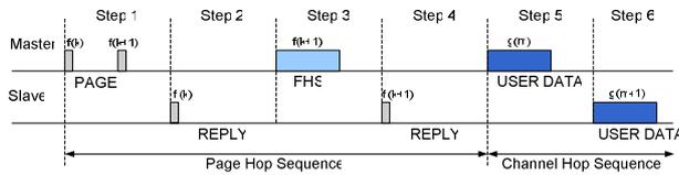
**Fig. 2: Connection establishment of two Bluetooth devices (master in page state and slave in page scan state).**
