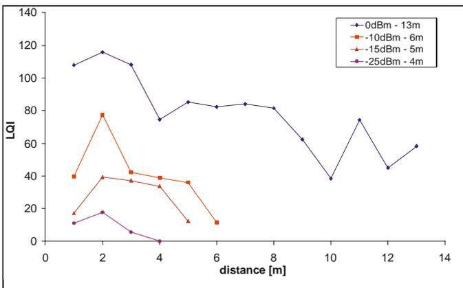
Figure 3. LQI vs. distance between two Zigbee-based sensor nodes (CC2420) in an indoor LSA environment for various transmission powers
