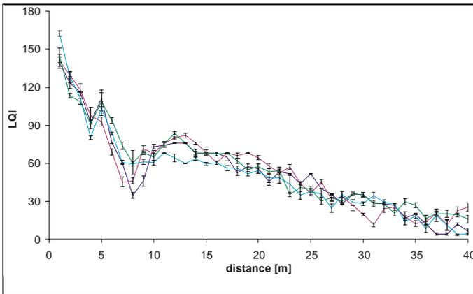
Figure 2. LQI vs. distance between two Zigbee-based sensor nodes (CC2420) in 20 loops in an outdoor environment. Each graph belongs to another sensor node
