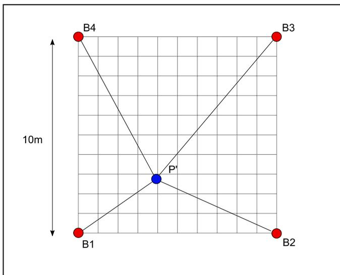
Figure 5. Testbed with 4 beacon nodes and 1 unknown node
