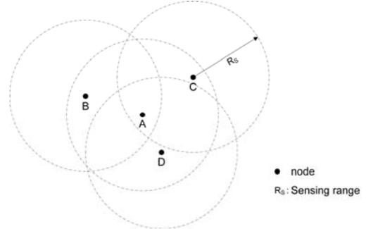
Fig. 4: Example for sensing redundancy of node A.
