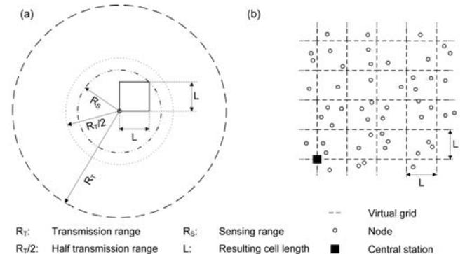
Fig. 5: (a) Cell size depends on sensing range (b) Visualization of resulting virtual grid
