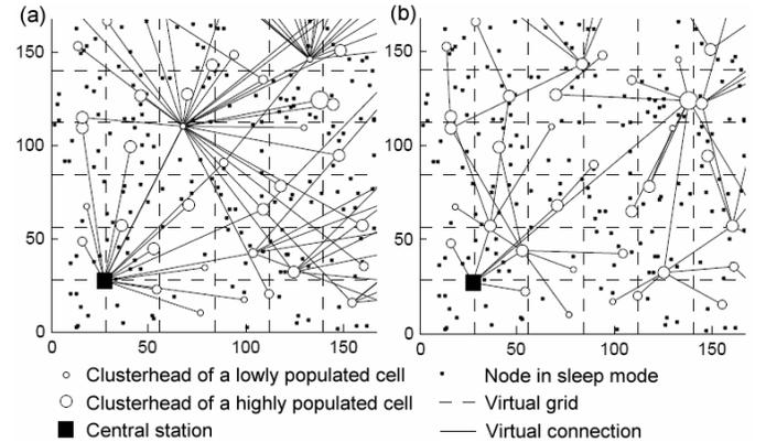
Fig. 7: Section of a large scale free network (a) without energy-awareness (b) with "Range Reduction", "Connectivity Limitation" and "Wait and See"
