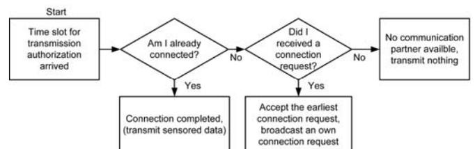
Fig. 1: Block diagram of the local algorithm on each node for scale free routing
