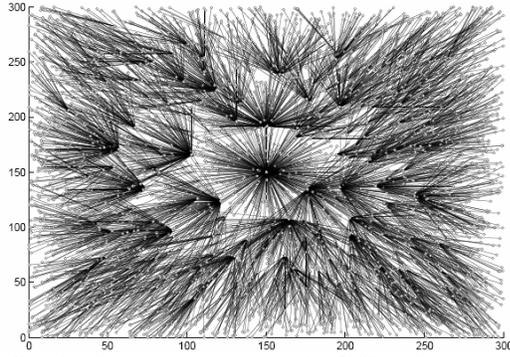
Fig. 2: Completed routing of a network. 5000 nodes were distributed randomly. Transmission range: 50m. Distribution area: 300m\*300m
