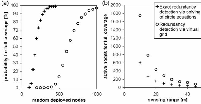
Fig. 6: Comparison of exact redundancy detection with our algorithm in a field of 300m\*300m (a) probability for full coverage of the area, transmission range=100m, sensing range=40m (b) estimation of necessary active nodes, transmission range=100m, deployed nodes = 5000
