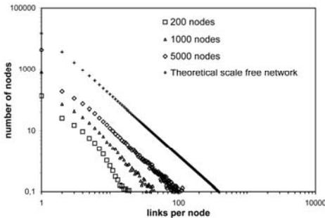
Fig. 3: Number of nodes versus number of links per node. Illustrated are our routing algorithm and a theoretical scale free network. Each result is averaged over 100 networks. Transmission range: 50m. Distribution area: 300m\*300m
