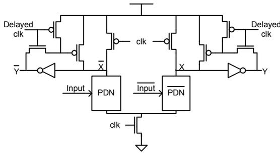
**Figure 3** Footed HS-Domino using extended keeper
