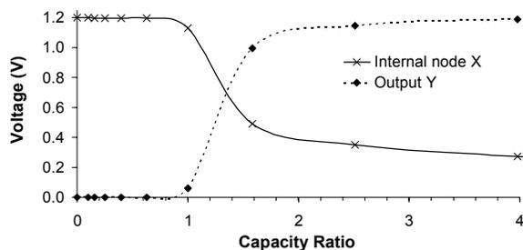
**Figure 7** Critical capacity ratio for charge sharing
