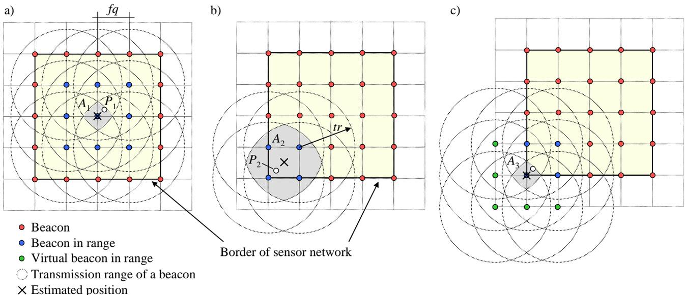
Fig. 2. Centroid localization in a grid based network of beacons a) in the center b) at an edge c) at an edge with virtual beacons
