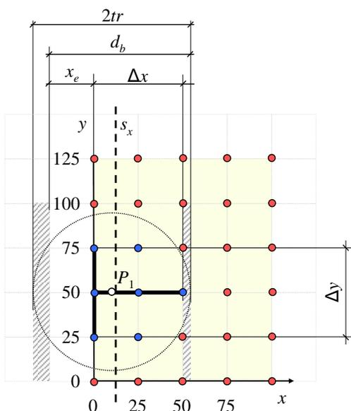
Fig. 3. Localization error of centroid localization
