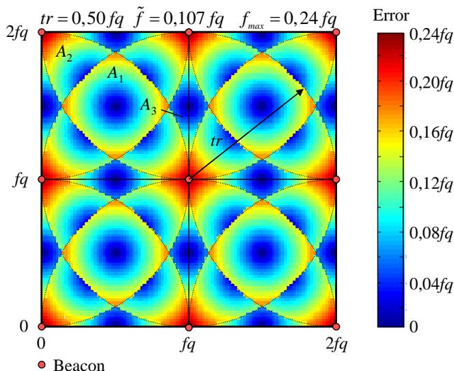
Fig. 1. Localization error of centroid localization
