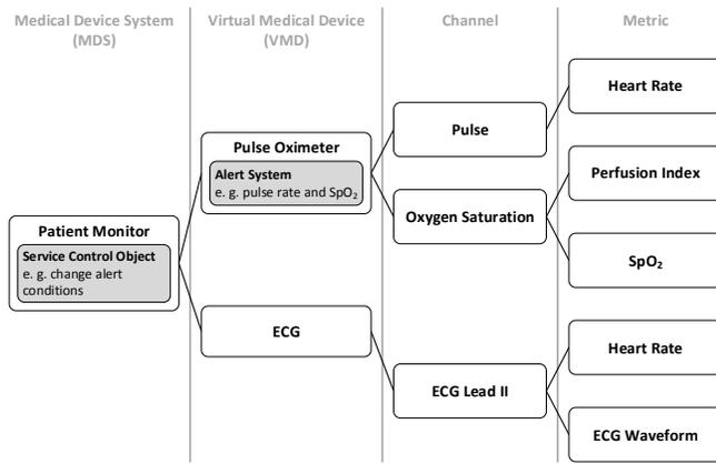
Fig. 2. Schematic overview of device capability modeling (containment tree for a simple patient monitor; note that a real patient monitor is much more complex than this example).
