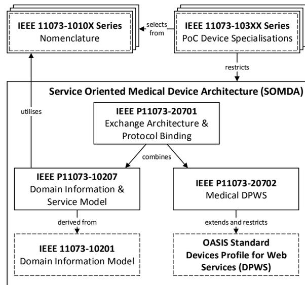
Fig. 1. Overview of considered standards and their relations. Dashed boxes indicate existing standards, solid boxes indicate new standards, and boxes with dashed and solid lines indicate existing standards that are being extended.
